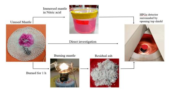
**Figure 2.** Three methods of mantle sample investigation: Direct; immersed in nitric acid; burned for 1 h.
