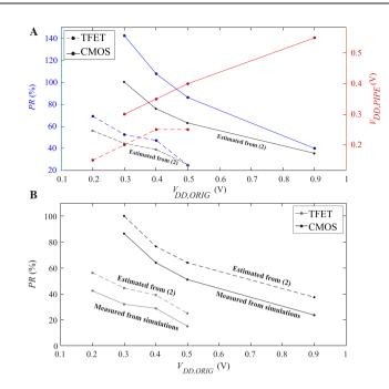
**FIGURE 4** A, *PR* (%) versus  $V_{DD,ORIG}$  and  $V_{DD,PIPE}$  versus  $V_{DD,ORIG}$  plots. B, *PR* (%) versus  $V_{DD,ORIG}$  without considering the impact of pipeline registers. TFET, tunnel field-effect transistor [Colour figure can be viewed at wileyonlinelibrary.com]
