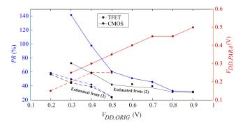
**FIGURE 3** *PR* (%) and  $V_{DD,PARA}$  versus  $V_{DD,ORIG}$ , including the *PR* (%) versus  $V_{DD,ORIG}$  estimation from expression 2. TFET, tunnel field-effect transistor [Colour figure can be viewed at wileyonlinelibrary.com]
