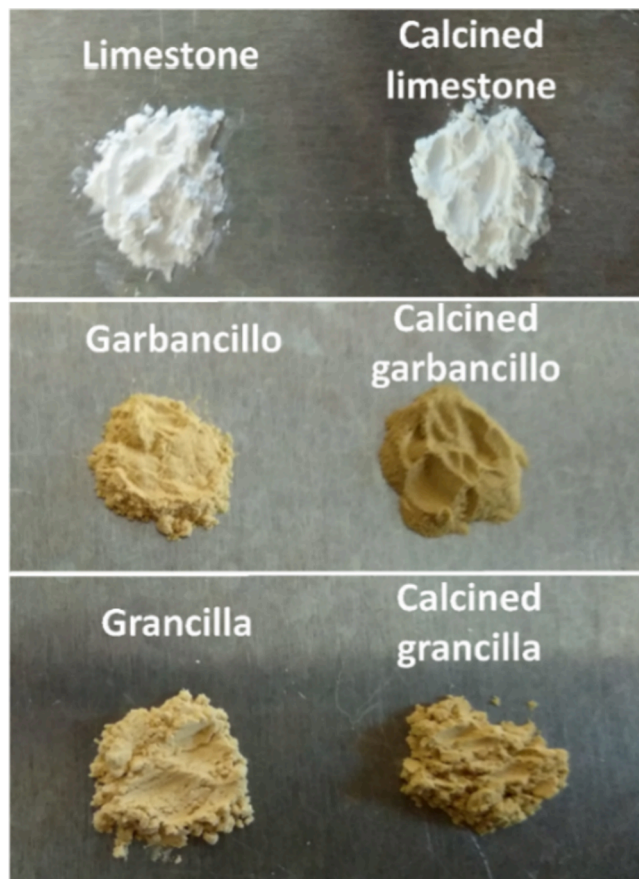
Fig. 4. Pictures of the samples of albero (before and after calcination) and limestone.
