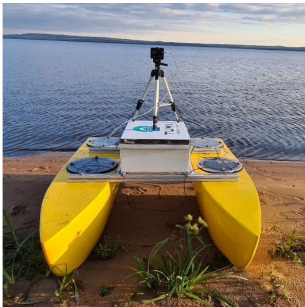
FIGURE 2. Example of an Autonomous Surface Vehicle for lake monitoring. Catamarans are usually the selected due to their enhanced stability.
