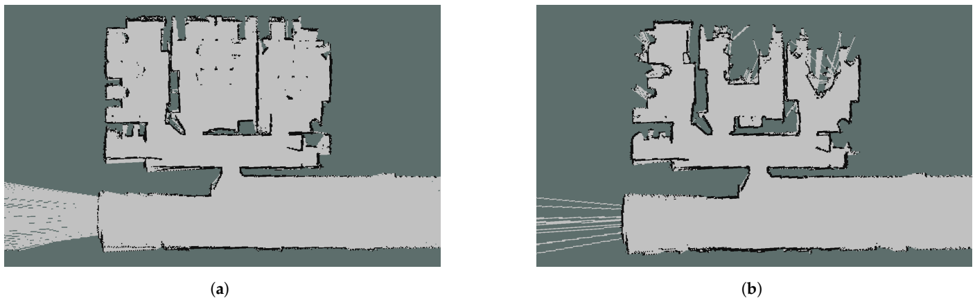
Figure 6. Map comparison between a pure 2D method and a traversable map where the height of the robot restricts the movement in certain areas such as under the tables. The results were obtained from a pre-recorded dataset [63] and default parameter values. The sensor is located at 60 cm of height, the resolution is of 0.4^\circ with an horizontal FoV of 360^\circ , the sensor frequency is 10 Hz and the robot height is 1 m: (a) resulting map given by Gmapping with a 2D LiDAR; (b) traversable (2.5D) map given by Gmapping using a 3D LiDAR and the Point-Cloud Fast Filter [70].
