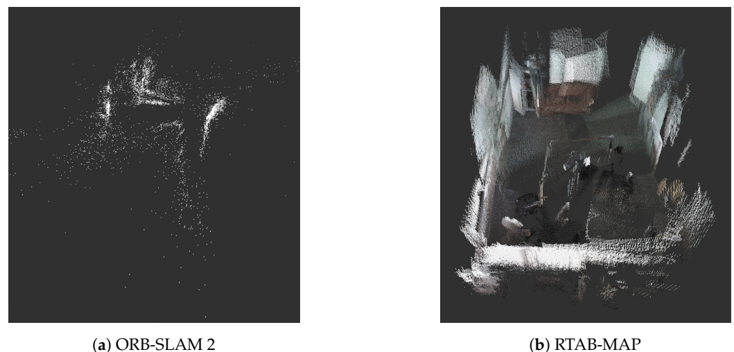
Figure 4. Resulting map for 3D SLAM algorithms using Orbbec Astra Pro camera data from a pre-recorded dataset [63] and the default parameter values (see Table 1 for the camera specifications). The camera was mounted on a Turtlebot 2 at 65 cm of height. The two figures have the same orientation.
