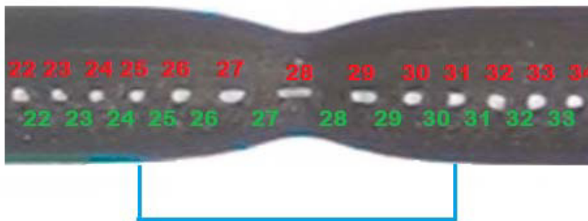
Fig. 6. Measured sections to determine the elongation at necking.
