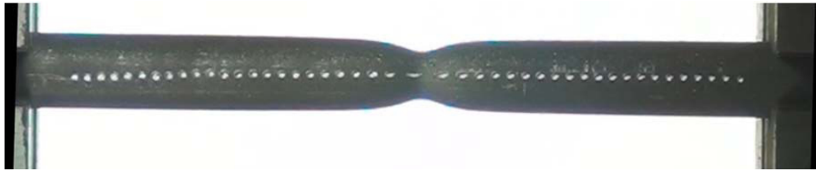
Fig. 3. Frame one of the specimens during the necking.
