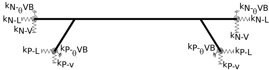
Figure 7: Schematic representation of the springs at foundations of the piers and abutments considered as updating parameters
