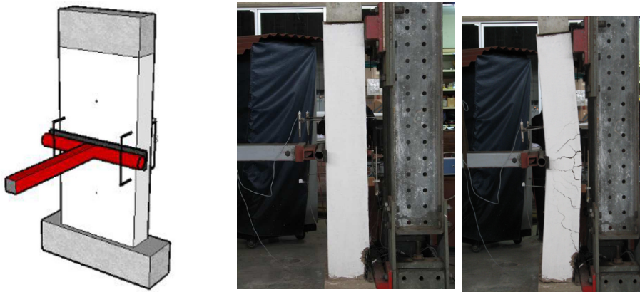
Figure 3. Three point bending tests of adobe walls
