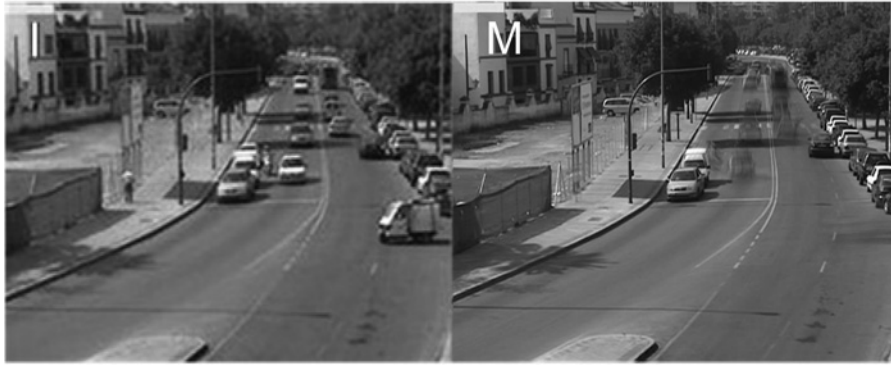
Fig. 3 Incorporation of stopped vehicles in front of a traffic light ( I : current frame, M : background model)
