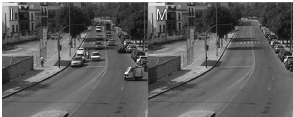
Fig. 6 Non-incorporation of stopped vehicles in front of a traffic light ( I : current frame, M : background model)
