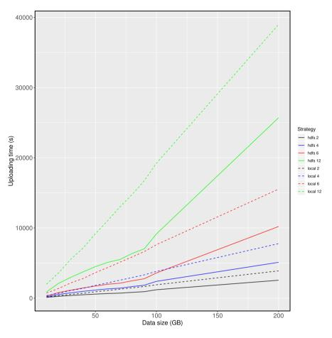
Fig. 4. Data uploading time evolution for local and HDFS strategies. (For interpretation of the colors in the figure(s), the reader is referred to the web version of this article.)
