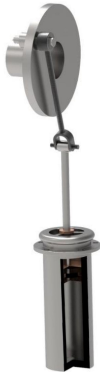
Figure 21. Juice pump subassembly.
