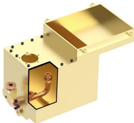
Figure 22. Juice collecting tank subassembly.
