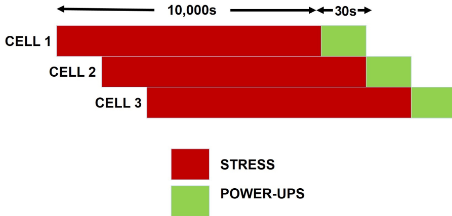
Figure 5.8: Schematic representation of the application of stress to the SRAM cells in a parallelized manner.
