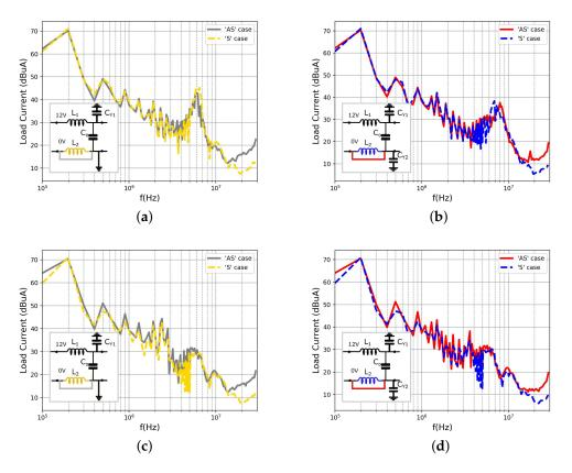
**Figure 8.** Measured DM output currents for symmetric ('S') and asymmetric ('AS') cases. (a)  $C_y = 10 \text{ nF. 'C0VG' configuration.}$  (b)  $C_y = 10 \text{ nF. 'CC' configuration.}$  (c)  $C_y = 50 \text{ nF. 'C0VG' configuration.}$  (d)  $C_y = 50 \text{ nF. 'CC' configuration.}$
