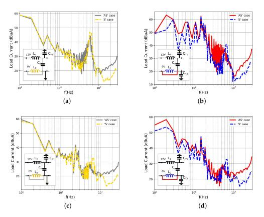
**Figure 6.** Measured CM output currents for symmetric ('S') and asymmetric ('AS') cases. (a)  $C_y = 10 \text{ nF. 'C0VG' configuration.}$  (b)  $C_y = 10 \text{ nF. 'CC' configuration.}$  (c)  $C_y = 50 \text{ nF. 'C0VG' configuration.}$  (d)  $C_y = 50 \text{ nF. 'CC' configuration.}$
