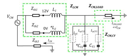
Figure 3. Simplified model of the CM path, depicted from the model in Figure 2.
