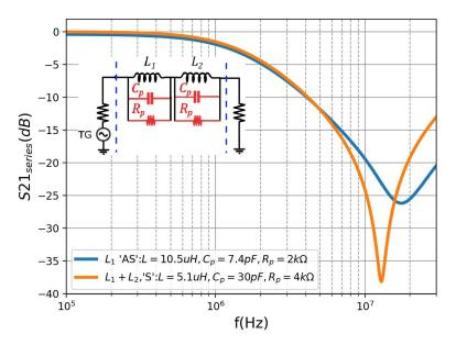
**Figure A2.** Transmission coefficient ( $S_{21}$ ) of the inductors  $L_1$  and  $L_2$  employed in 'S' and 'AS' configurations of the output LC filter of the converter.
