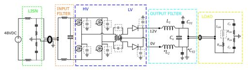
**Figure 1.** PSFB topology schematic. Paths that account for CM emissions are also represented.  $*C_{Y2}$  accounts either for a direct bonding connection or for a capacitive coupling to the converter grounded chassis.
