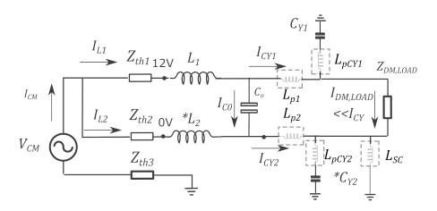
**Figure 4.** Model to predict CM to DM conversion in the proposed filter configurations, derived from the circuit model in Figure 2.
