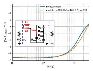
**Figure A1.** Measured and simulated transmission coefficient  $S_{21}$  of the shunted CM load with the cables.
