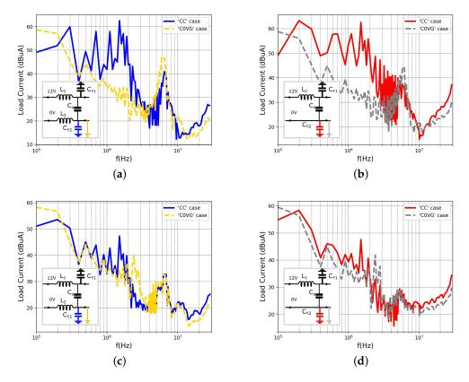
**Figure 7.** Measured CM output currents for 'C0VG' and 'CC'. (a)  $C_y = 10$  nF, 'S' case. (b)  $C_y = 10$  nF, 'AS' case. (c)  $C_y = 50$  nF, 'S' case. (d)  $C_y = 50$  nF, 'AS' case.
