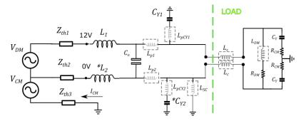
**Figure 2.** Equivalent model of the converter at the output. In 'S' configurations:  $L_1 = L/2$ ,  $L_2 = L/2$ . In 'AS' configurations:  $L_1 = L$ ,  $L_2 = 0$ . In 'CC' configurations:  $C_{Y1} = C_Y$  and  $C_{Y2} = C_Y$ . In 'C0VG' configurations:  $C_{Y1} = C_Y$  and  $C_{Y2}$  is a short circuit. Asterisks in  $L_2$  and  $C_{Y2}$  indicate that these components might not be present depending on the filter configuration.
