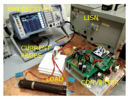
Figure 5. Experimental setup for measuring conducted emissions at the output leads of the converter.
