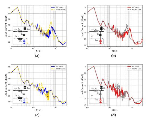
**Figure 9.** Measured DM output currents for 'C0VG' and 'CC'. (a)  $C_y = 10$  nF, 'S' case. (b)  $C_y = 10$  nF, 'AS' case. (c)  $C_y = 50$  nF, 'S' case. (d)  $C_y = 50$  nF, 'AS' case.
