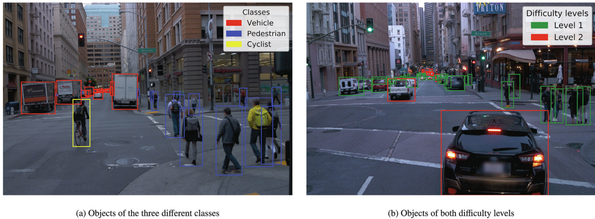
Fig. 2. 2D object detection problem in the Waymo Open Dataset.
