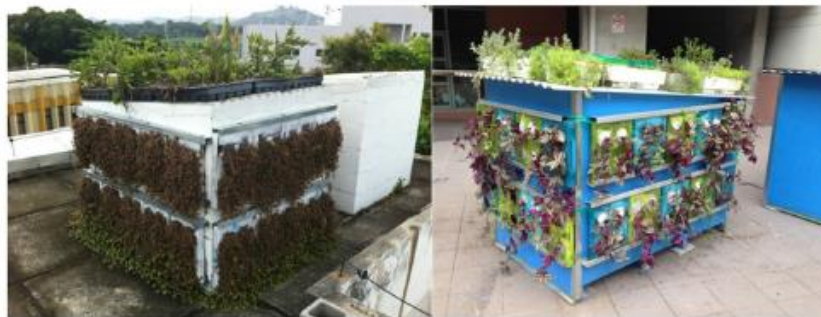
Fig. 1. Green roof and green walls experimental setup. Left-hand side – Rio de Janeiro, right-hand side – Sydney. (For interpretation of the references to colour in this figure legend, the reader is referred to the Web version of this article.)
