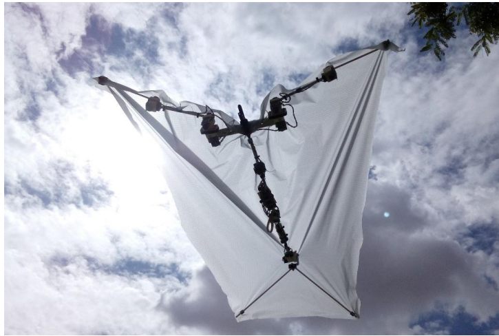
Figure 1. Prototype of winged aerial manipulation robot with dual arm and tail.
