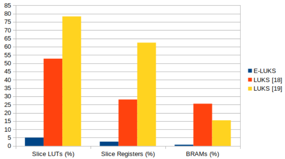
Figure 6. Percentage resources of E-LUKS and LUKS solutions for the XC7Z020 FPGA.
