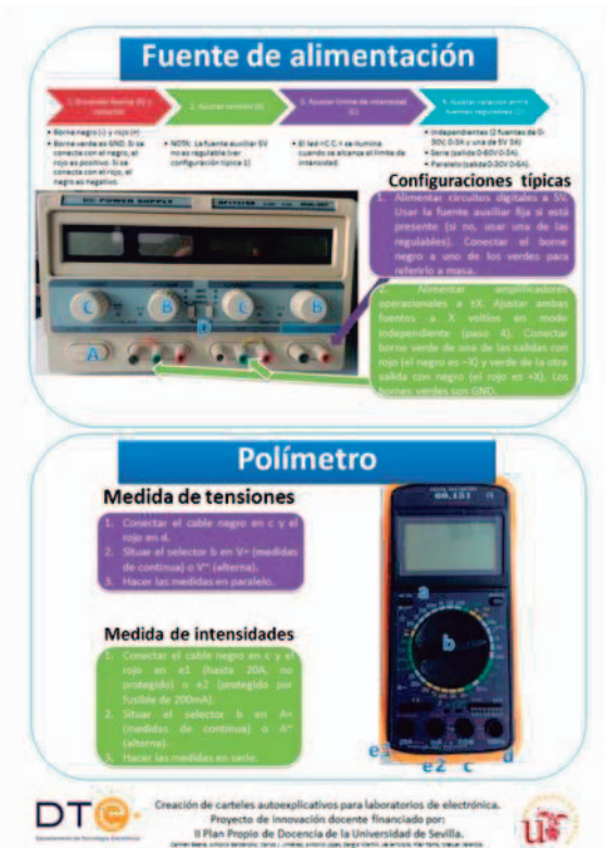
Figure 1: Poster 1: Multimeter and DC Power Supply
