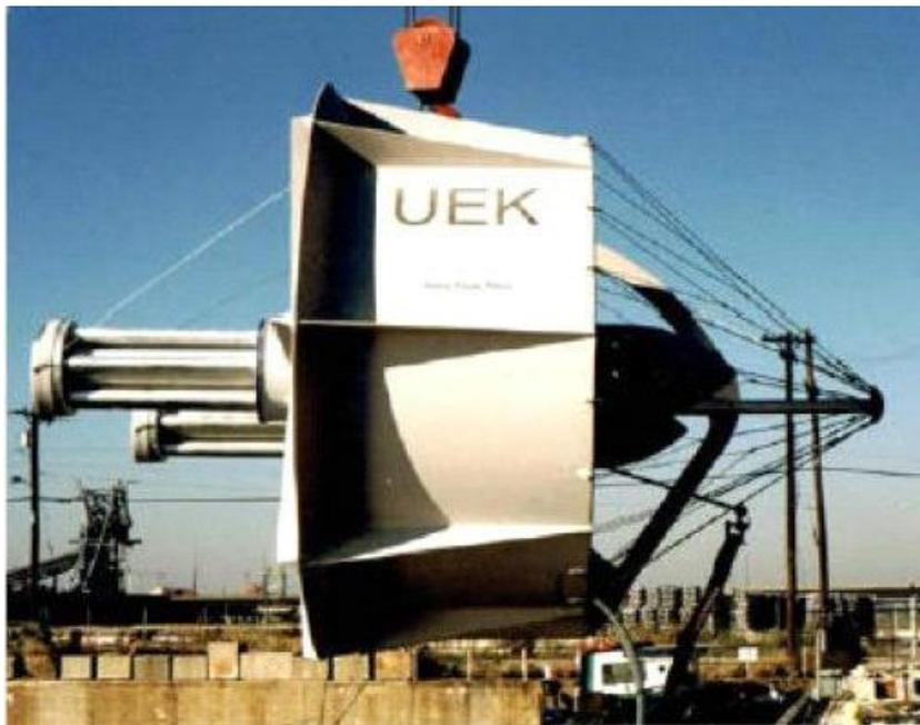
Figura 5-7. Turbina Underwater Electric Kite
