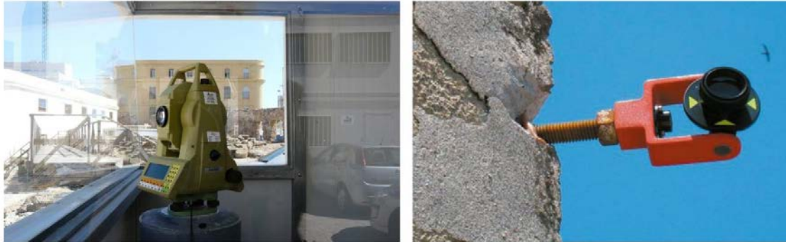
Fig. 7. Total station of topographical control (left). Target (right).
