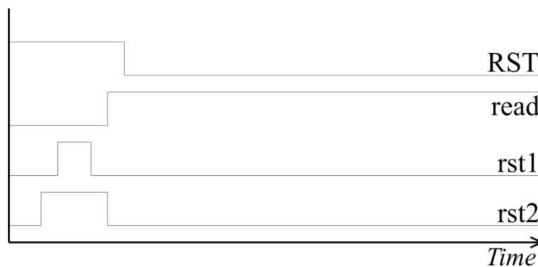
Fig. 33: Timing diagram of the autozeroing comparator.
