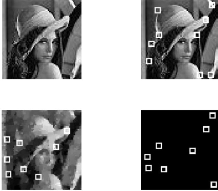
Fig. 58: (Top Left) Original Image; (Top right) Original image with Harris; (Bottom left) NESTA reconstructed image with Harris; (Bottom right) Harris NESTA corners.
