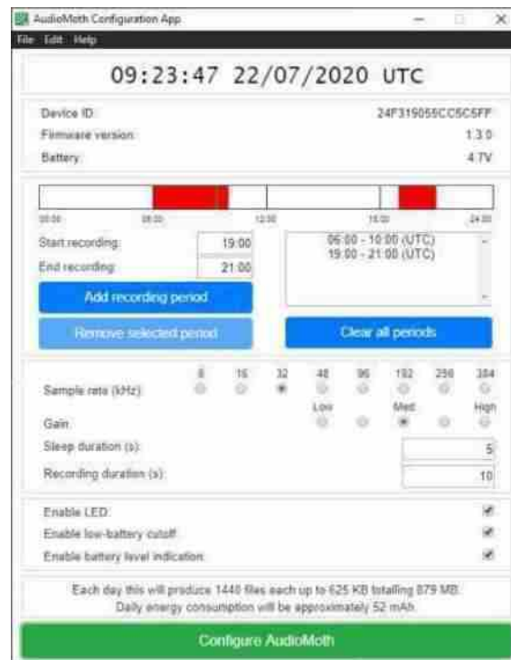
Figure 3.3: Configuration example in AudioMoth Configuration App. Two recording periods are selected, as well as sample rate, gain, recording and sleep duration. At the end, the app informs about the number of files produced, their size and daily energy consumption.
