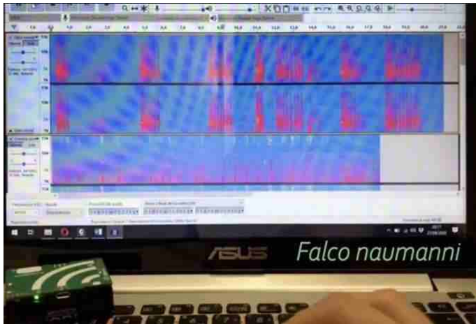
Figure 3.12: System operating test. AudioMoth is recording and it has detected a vocalization of F. naumanni . Consequently, the green LED (bottom left corner) has been activated.
