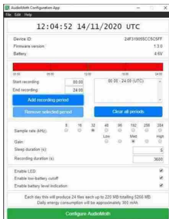
Figure 3.16: Configuration of a recording period of 24 hours. The energy consumption is shown above 'Configure AudioMoth' button.
