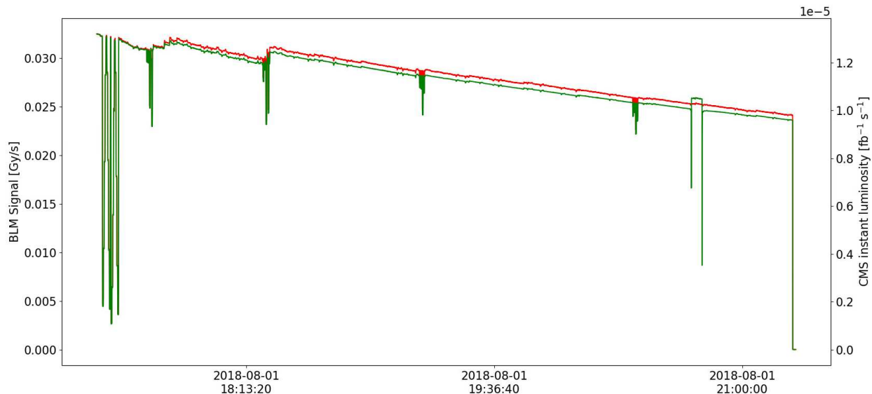
Figure 18: BLM signal of a detector located near IP5 and instant luminosity in CMS during a STABLE beam mode period. The BLM signal is indicated in red and the instant luminosity in green.
