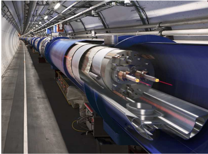
Figure A.2: LHC tunnel and 3D recreation of the inner part of a dipole (bending) magnet and the beam pipes. The section of the beam pipes is indicated in yellow, and the circulating beams are indicated in red [36].
