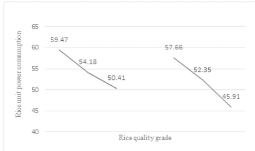
Fig. 3. Evaluation standard value of unit electricity consumption of 225 japonica in the rice processing loss evaluation system
