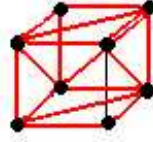
Figure 5.13: Example showing one possible selection of the diagonals for each face of the cube. This selection gives rise to a concrete tetrahedralization of the cube.
