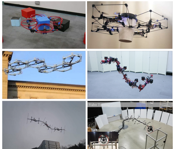
Fig. 5: Examples of interconnected actuated multi-body designs (from top, from left): 1) HYDRUS [105]; 2) flying-gripper [146]; 3) distributed flight array (DFA) [147]; 4) DRAGON [148]; 5) flying LASDRA [149]; and 6) operation LASDRA [109].
