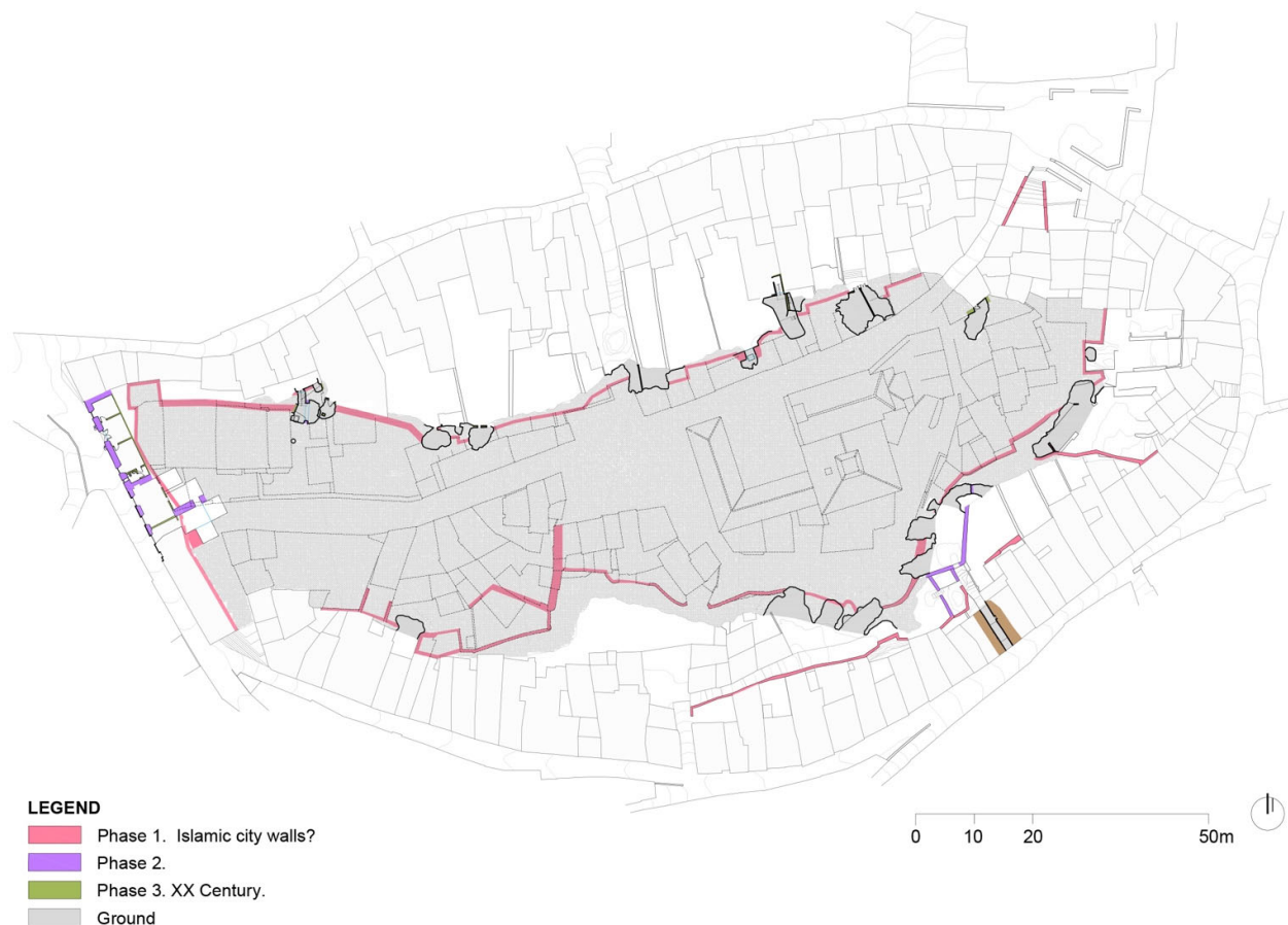
Figure 18. Floor level -1. Large number of caves and cavities existing under the walled enclosure that have been discovered and can be observed after the photogrammetric survey [authors' own drawing].
