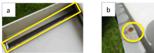
Fig. 2. Frame defects: silicone joint cracked (a) and grounding screw oxidation (b).
