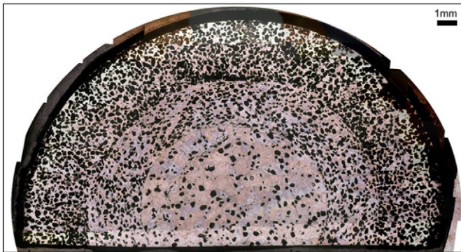
Fig. 5. Assembly of 120 optical microscope images showing a top view of a radial cross-section, and after polishing of a sintered Ti cylinder, showing the three different zones (core, inner shell and outer shell).
