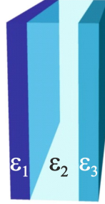
Figure 1.4: Scheme of a plane-parallel system with a material (that might be different from vacuum) between the interacting bodies.
