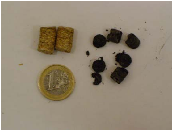
Figure 8: Virgin corn stover pellets and the char obtained from devolatilization of these pellets in fluidized bed
