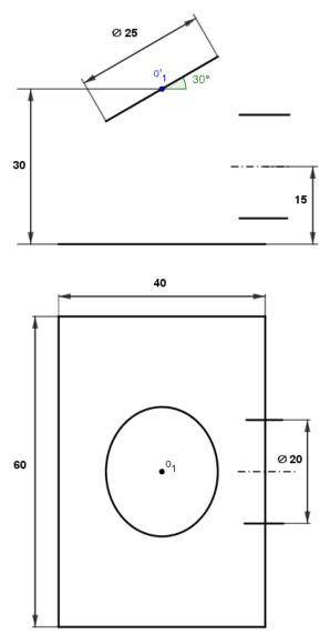
**Figure 3.** Orthographic views with reference dimensions (cm) of transformer sections with round cylindric branch (see text).
