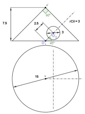
**Figure 1.** Orthographic views with reference dimensions (m) of the four-way cylindric hopper to be built, where the wrapping cone intersecting the cylinder defines the upper border or junction (see text).
