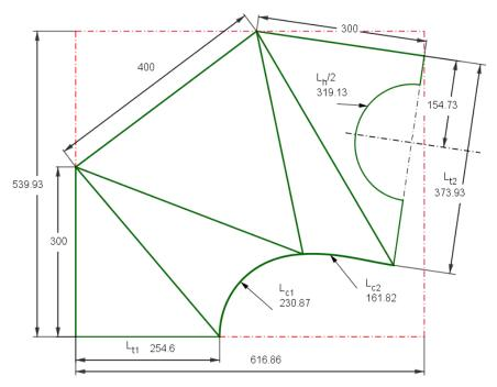
**Figure 8.** Dimensioned (mm) half-pattern of the Round-poligonal transformer with circular branch obtained by the CEDG approach with 120 generatrix lines for the reference parameters' values.
