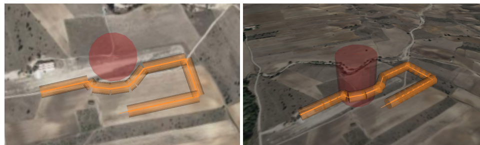
Figure 19. A top (left) and a perspective (right) view of the optimal solution in the use case 2. An alternative flight plan for UAS 2 is generated to avoid the geofence.
