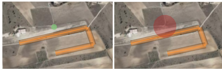
Figure 18. (Left), top view with the initial flight plans in the use case 2. The Operational Volumes without conflicts are also shown. (Right), situation after the detection of the jamming attack. A geofence (in red) is created around the attacked UAS, which generates a conflict with the flight plan of the other UAS.
