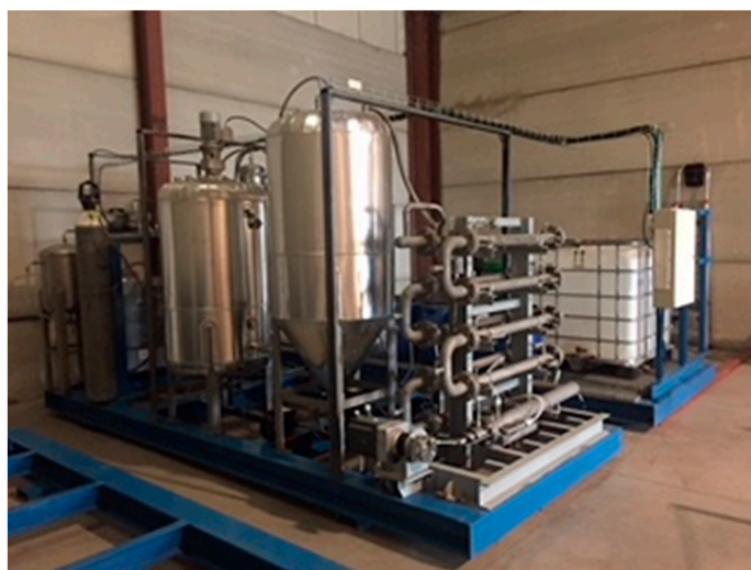
Figure 1. Pilot plant for the production of the biodiesel and glycerin used in this research.
