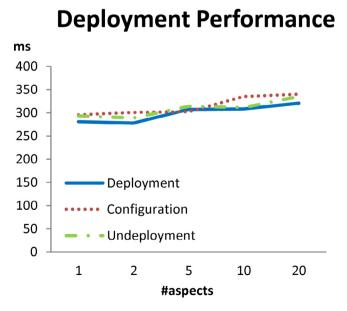
Fig. B4 – Performance of deploying, reconfiguring, and undeploying security policies.
