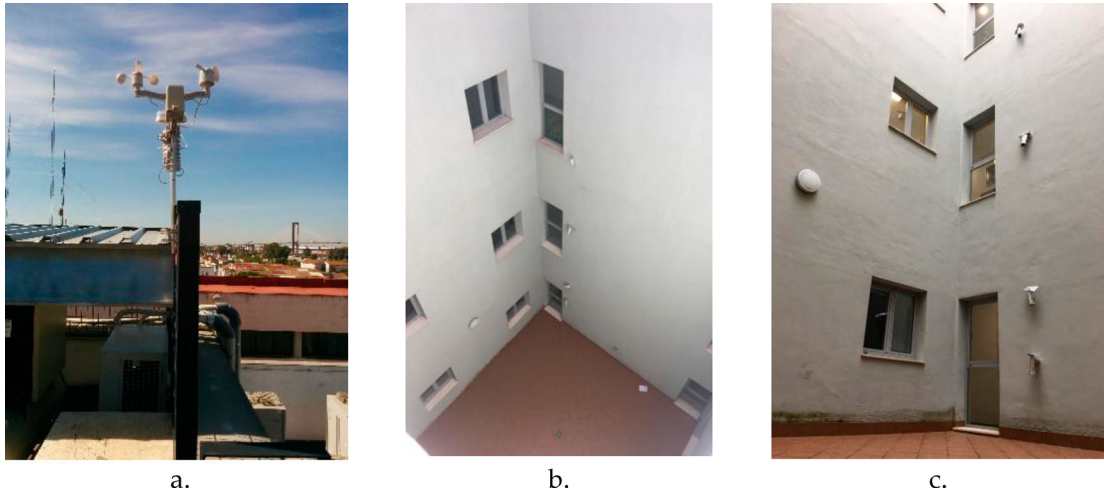
Figure 6. Images of the measuring instruments placed at the case study. a. Weather Station at the roof. b. Temperature and relative humidity sensors. Top view. c. Temperature and relative humidity sensors. Bottom view.
