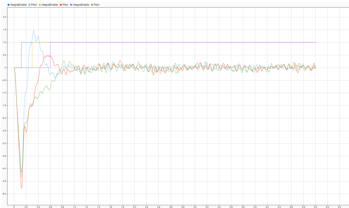
Figure 4-17. Pitch angle response when delaying too much the integral component of the PID (in blue)
