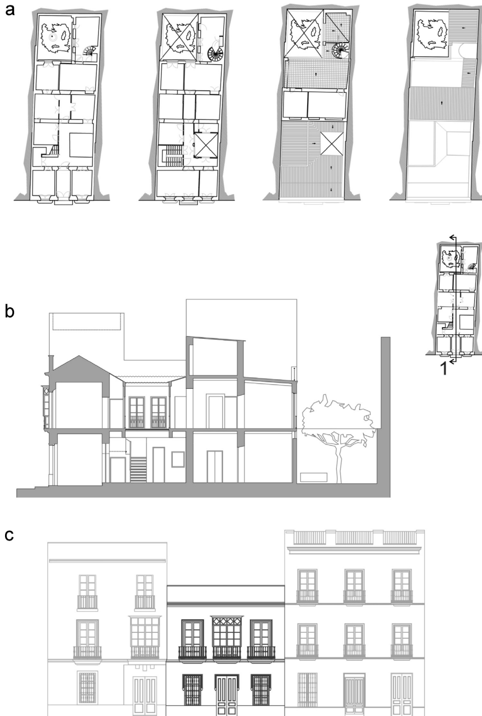
Fig. 1. Model A. (a) Plans, (b) Section 1 and (c) elevation.
