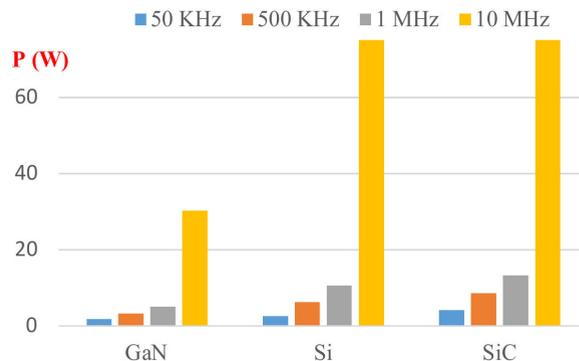
FIGURE 8. Average power dissipation of each transistor (GaN, Si, SiC) for different frequencies.
