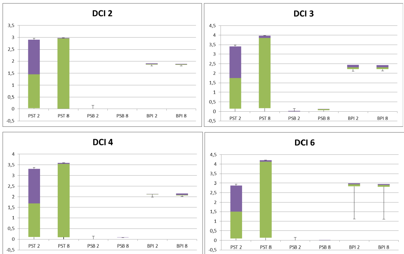
Figure 8. Distribution of PSNR drops (y-axis), with respect to CIBO strategy, for each method applied with 2 and 8 GOP (e.g. PST 2 is the method PST in 2GOP), to the four sequences tested in the experiment.
