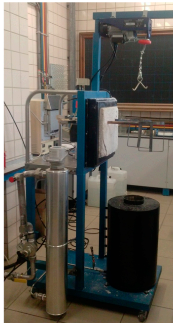
Figure 7. Complete metal spheres packing device for energy recovery.
