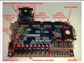
Figure 2. Prototyping board to be used during the lab session
