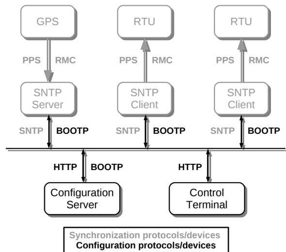
**Fig. 1.** Typical scenario for deploying hardware SNTP client and servers (synchronization devices and protocols are marked in gray, and configuration devices and protocols are marked in black).
