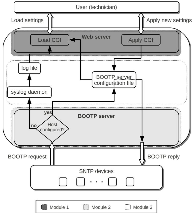
**Fig. 3.** Overall diagram of the configuration server operation.
