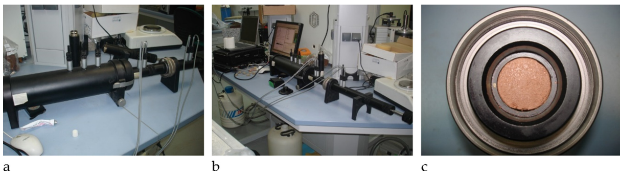
Fig. 4. a) and b) Test setup with the impedance tube kit. c) Test sample placed inside the tube.
