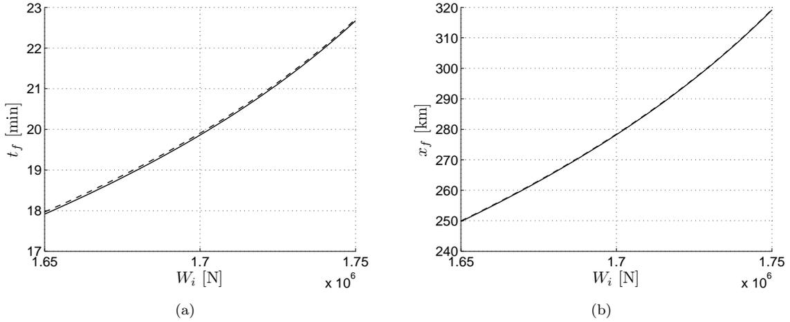
Figure 4: Flight time (a) and Range (b) vs. initial aircraft weight. Solid lines: optimal climb. Dashed lines: optimized CAS-Mach climb.
