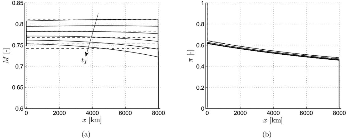
Figure 6: Trajectories (a) and control (b) for different arrival times ( $t_f = 9.17, 9.33, 9.5, 9.67, 9.83, 10$  h,  $h = 10000$  m,  $W_i = 1600$  kN). Solid lines: optimal cruise. Dashed lines: constant-Mach cruise.
