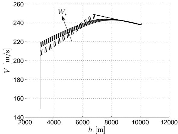
Figure 1:  $V(h)$  comparison for  $W_i = 1650, 1675, 1700, 1725$  and  $1750$  kN. Solid lines: optimal climb. Dashed lines: optimized CAS-Mach climb.
