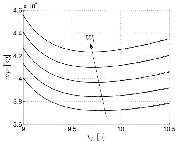
Figure 7: Minimum fuel consumption vs flight time, for  $W_i = 1500, 1550, 1600, 1650, 1700$  kN ( $h = 10000$  m). Solid lines: optimal cruise. Dashed lines: constant-Mach cruise.
