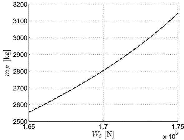
Figure 3: Minimum fuel consumption vs. initial aircraft weight. Solid lines: optimal climb. Dashed lines: optimized CAS-Mach climb.
