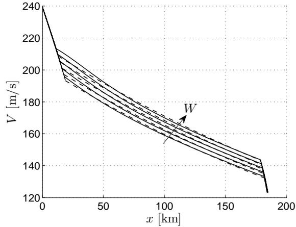
Figure 8:  $V(x)$  comparison for  $W = 1100, 1150, 1200, 1250$  and  $1300$  kN. Solid lines: optimal descent. Dashed lines: optimized constant-CAS descent.
