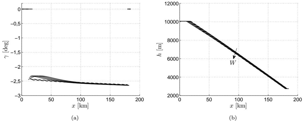
Figure 9:  $\gamma(h)$  and  $h(x)$  comparison for  $W = 1100, 1150, 1200, 1250$  and  $1300$  kN. Solid lines: optimal descent. Dashed lines: optimized constant-CAS descent.
