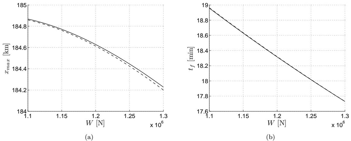
Figure 10: Maximum range (a) and flight time (b) vs. aircraft weight. Solid line: optimal descent. Dashed line: optimized constant-CAS descent.
