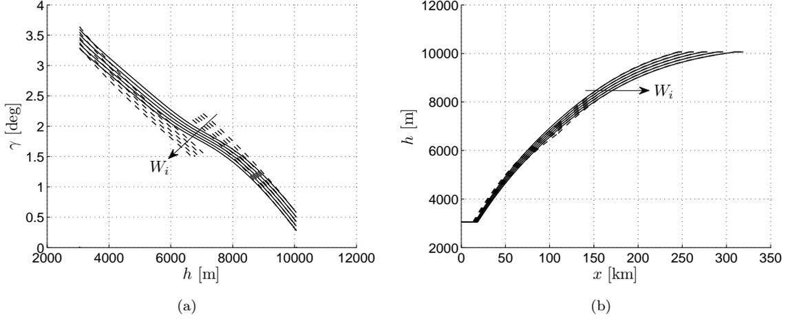
Figure 2:  $\gamma(h)$  and  $h(x)$  comparison for  $W_i = 1650, 1675, 1700, 1725$  and  $1750$  kN. Solid lines: optimal climb. Dashed lines: optimized CAS-Mach climb.
