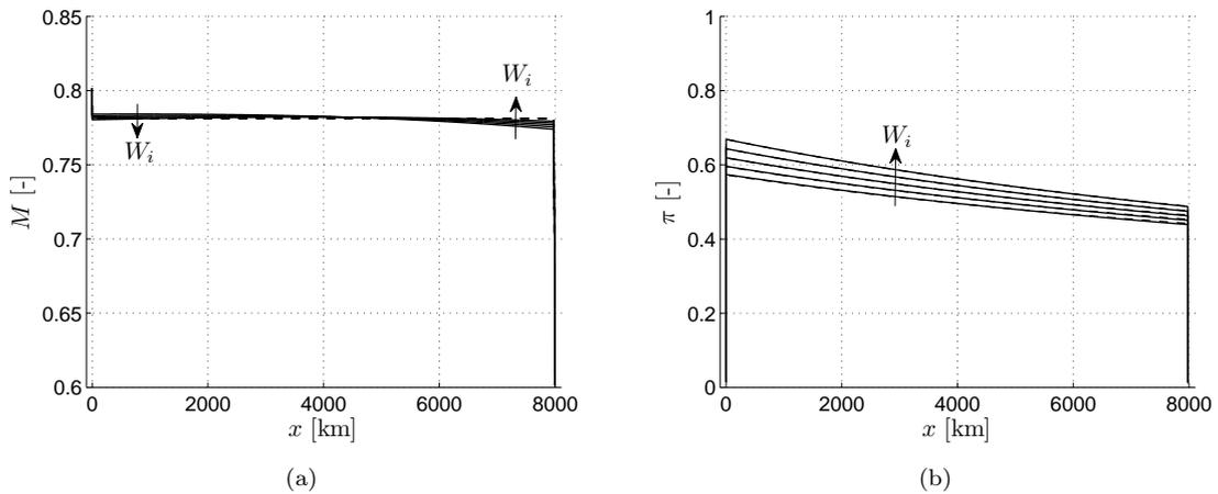
Figure 5: Trajectories (a) and control (b) for  $W_i = 1500, 1550, 1600, 1650, 1700$  kN ( $t_f = 9.5$  h,  $h = 10000$  m). Solid lines: optimal cruise. Dashed lines: constant-Mach cruise.
