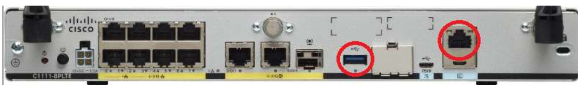
Figura 3-22. Router Cisco C1111-8P indicando puerto USB y consola.
