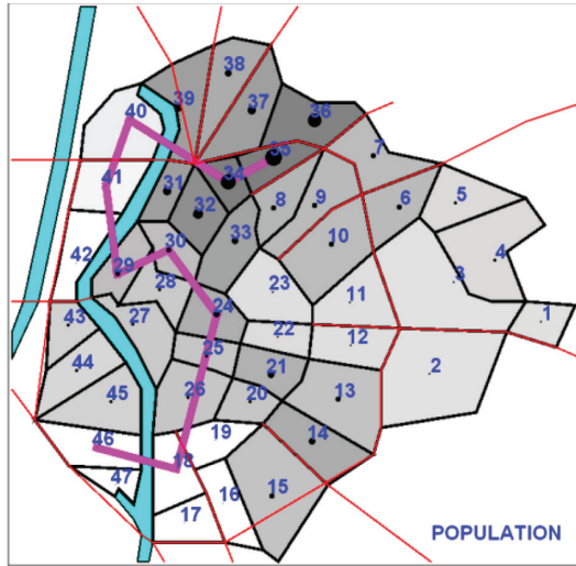
Figure 4: 9-station line obtained for the criterion of maximizing the global urban entropy.
