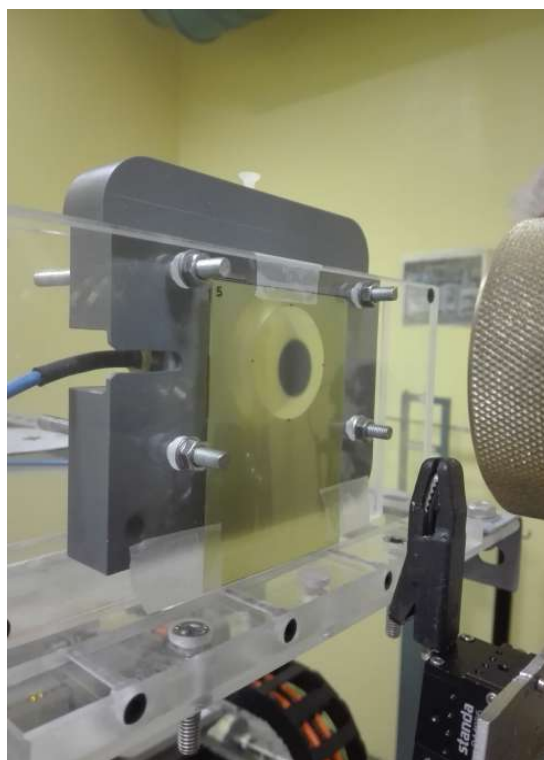
Figure 2.9: Example of a setup for the measurement of the beam profiles. A piece of EBT3 film is placed at a distance of 10.9 cm from the exit flange (configuration B.2 in Table 2.4).
