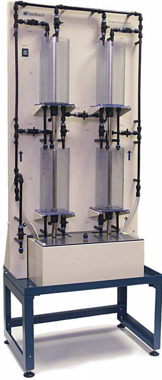
Figure 2: Plant of four-coupled tanks.
