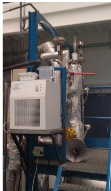
Figura 9. Reactor "Steam Explosion"
